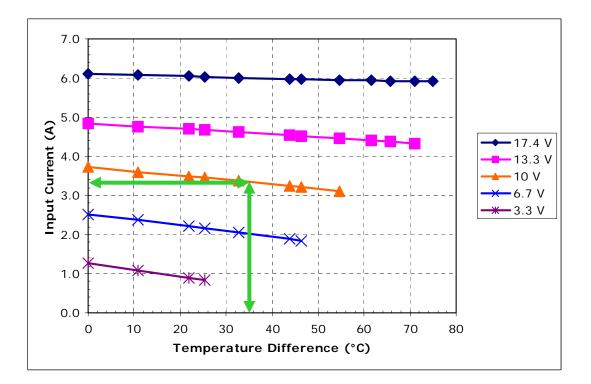
Once you know the input voltage, you can then determine what the steady-state current draw the module will have. In the example, a vertical line is drawn from the "Temperature Difference" axis until it intersects the graphed line representing the input voltage. Then draw a horizontal line from the intersection to "Input Current" axis to determine the current draw.
