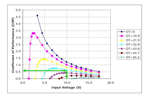
As with the heat removed in our current example, we have also already determined that the coefficient of performance (COP) is 0.6 [20 W of cooling divided by (10 V x 3.3 A) power input, 20/33 = 0.6]. However, this graph provides a visual indication of how far off of the maximum COP that the operating point is.
