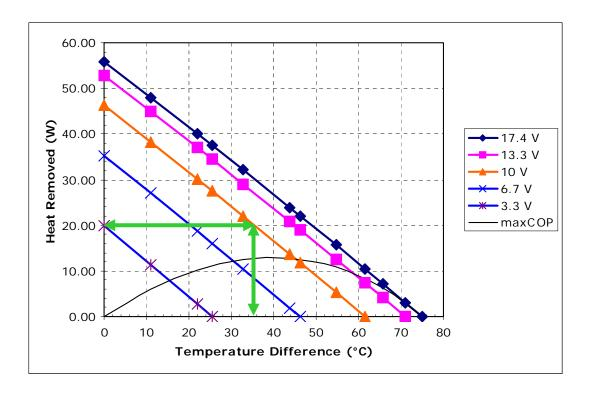
If you know the amount of heat load you need to remove and the desired cold-side temperature, you can determine what input voltage is required. Suppose you need to remove 20 W of heat at 15 °C and assume for now that the hot side of the module is at 50 °C. The temperature difference is then 50 -15 = 35 °C. Therefore, the module would need a 10 V input.
