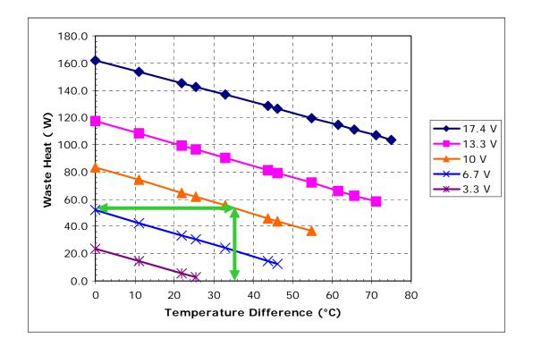
With our current example, we have actually already determined that the waste heat is 53 W (20 W of cooling plus 10 V x 3.3 A power input = 53 W). However, if you already knew the thermal resistance of your heat sink but did not know how much heat you could remove from the cold side, you could use this graph as your starting point.
